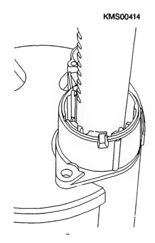
Checking drive-end bearing
